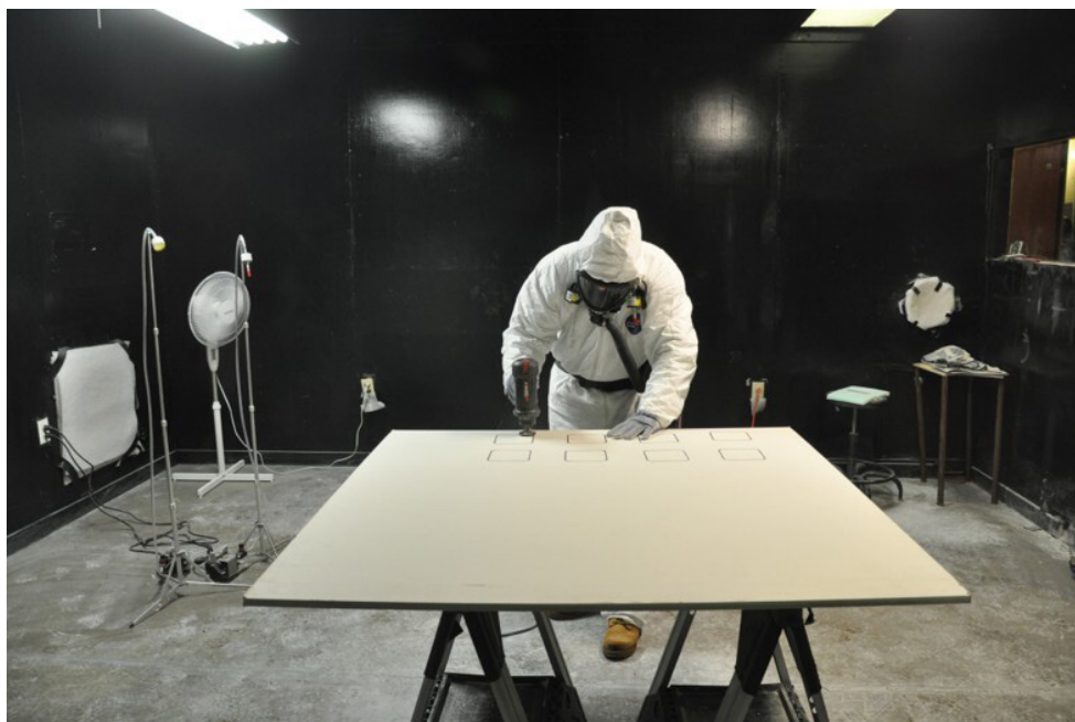
Illustration of personal and area air sampling for airborne particulates while a worker is cutting construction materials within a test chamber.
