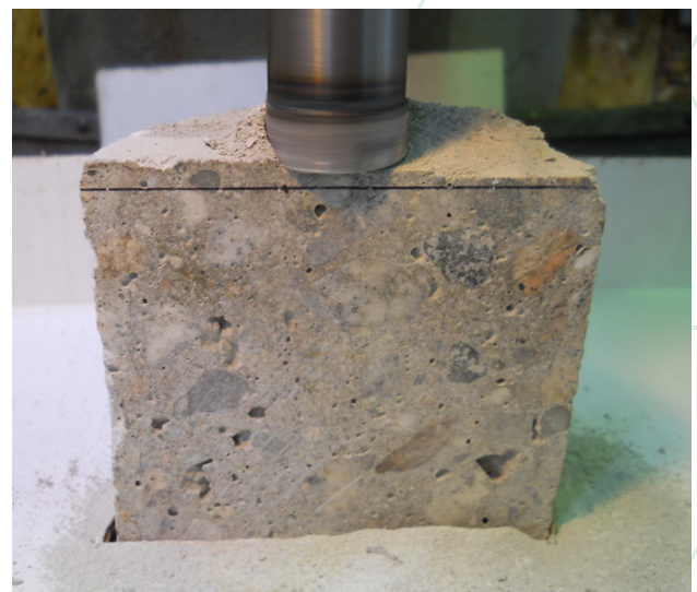
Photograph of milling the surface of a concrete half-core to extract sample for acid-soluble chloride.
